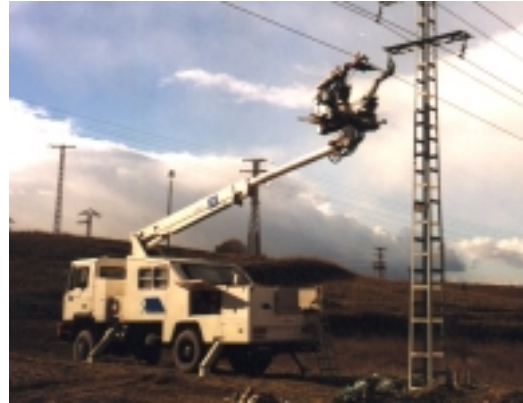
Figure 1. General view of the ROBTET
